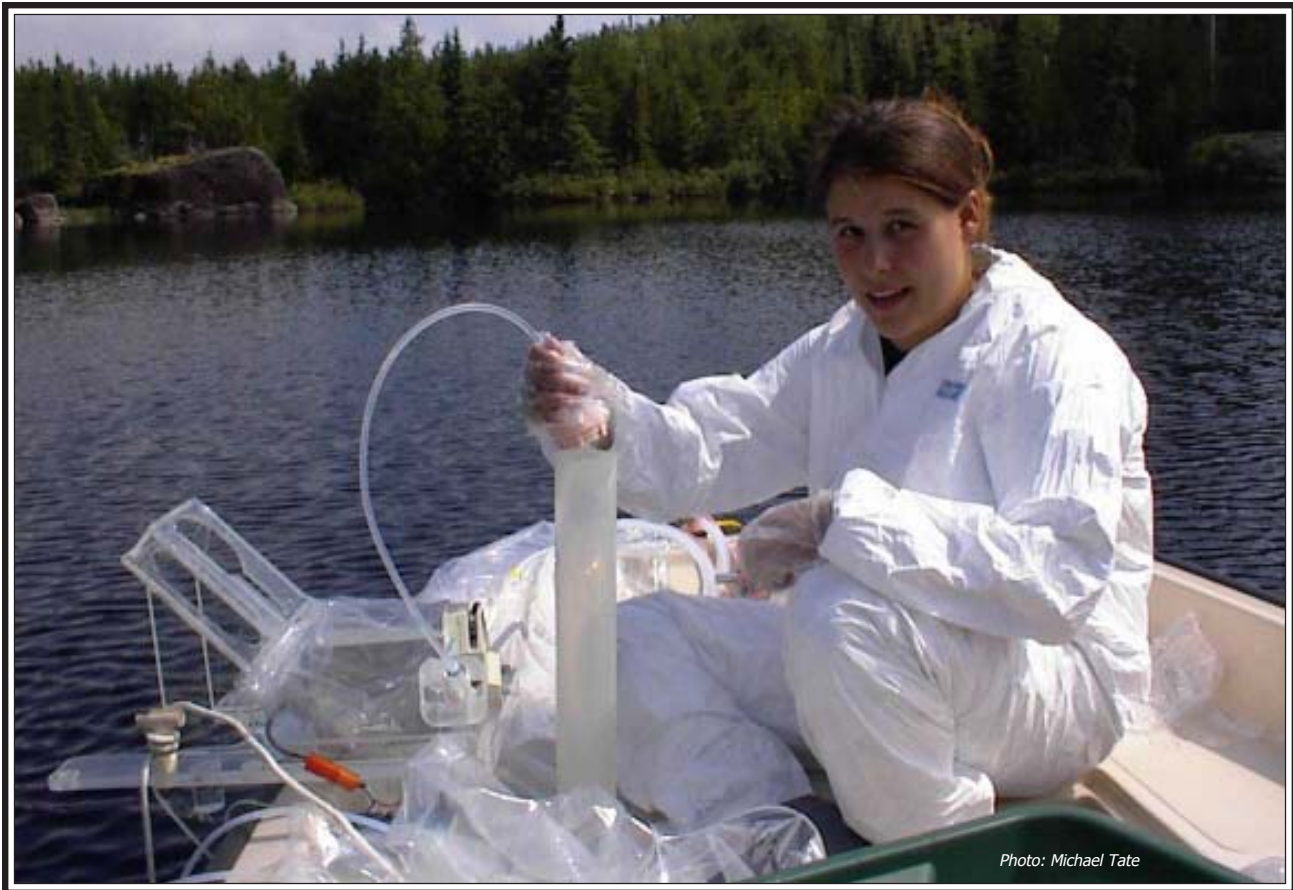
Tara Trinko, a technician from Wisconsin, samples Lake 658 for mercury content. The mercury levels are so low that samplers must wear "clean" clothing and gloves to avoid introducing any contamination that would ruin the samples.
