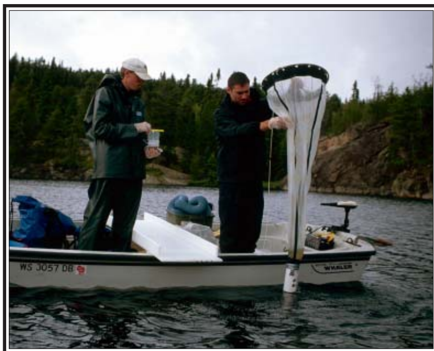
Justin Shead and Ken Sandilands sample microscopic animals (zooplankton) from Lake 658, the site of the METAALICUS study. The whole ecosystem is being carefully monitored to detect the presence and movement of mercury. (Photo by Karen Scott)
